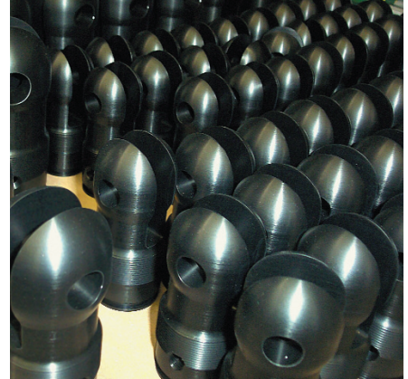
For this 6xxx alloy marine application, hardcoat anodizing was followed by post treatment (sealing).
