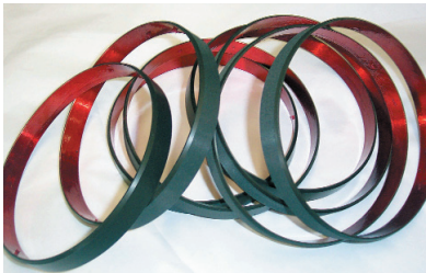
These 2xxx alloy rings were hardcoat anodized for an aerospace application; the red is masking.
