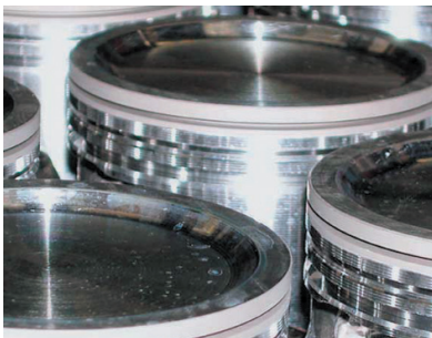
These pistons were hardcoat anodized to minimize the microwelding effect that can occur in the ring groove when pistons reach high temperatures.
