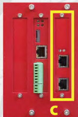
Profinet (c) Ethernet-IP (c) Modbus/TCP (c)
