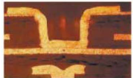
0.009" x 0.009" blind via (230 x 230 μm)
